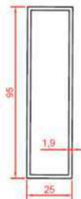
SB 21516 95X25 Louvre profile 1.225 kg/m
